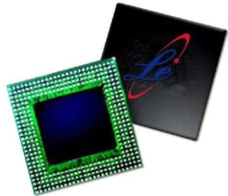
The content processor is implemented in deep sub-micron semiconductor technology. It consists of five major units: packet pre-processing, protocol parser, policy-based classifier, packet modification and forwarding engine, and system interface functions (See Figure 1).
